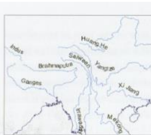
Figure 3.50 Line labels placed automatically by ArcMap. Source: Digital Chart of the World, ESRI.
